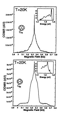
**Figure 2.** The full-field X-band total PL-ODMR of (a)  $C_{60}$  and (b)  $C_{70}$  films at 20 K. Insets: The respective PL spectra.
