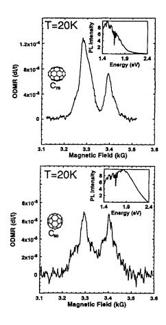
Figure 1. The full-field X-band total PL-ODMR of (a)  $C_{60}$ :T/PS and (b)  $C_{70}$ :T/PS glasses. Insets: The respective PL spectra.
